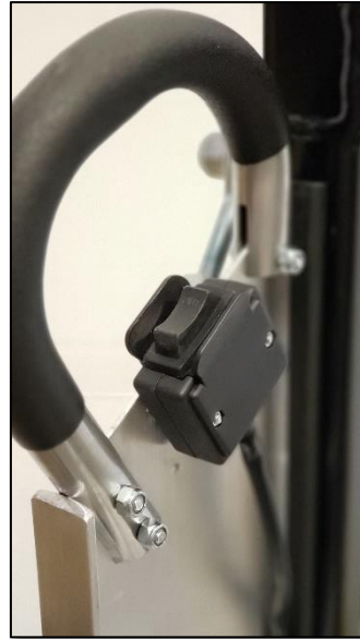
FIG. 8.2 ELECTRIC WINCH SWITCH
