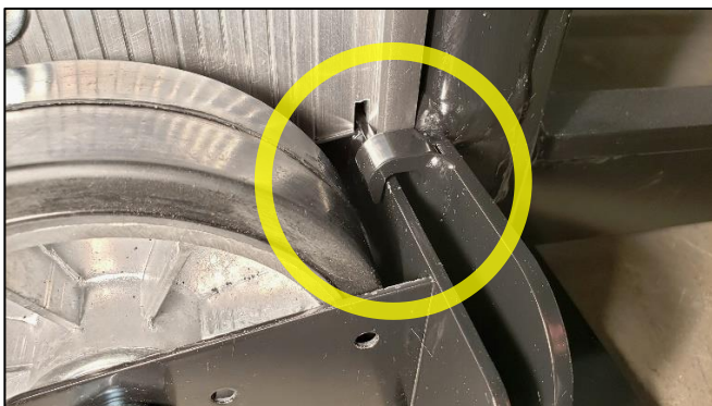
FIG. 9.2 – LIFT FRAME TOE HOOK SECURED OVER TOE PLATE
