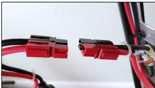
FIG. 4.1 – BATTERY HARNESS QUICK CONNECTORS
