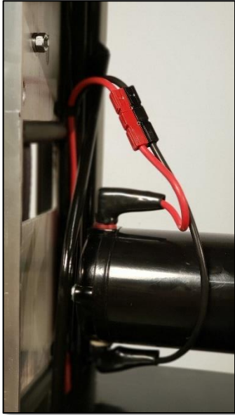
FIG. 8.1 ELECTRIC WINCH QUICK-CONNECTOR FOR REMOVABLE LIFT FRAME
