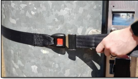
FIG. 6.1 – TIGHTENING THE SAFETY STRAP
