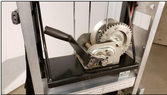
FIG. 9.1 – HAND WINCH HANDLE FOLDED INTO FRAME
