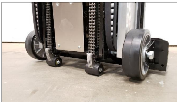
FIG. 10.2 – LIFTING FEET USED AS A PARKING BRAKE
