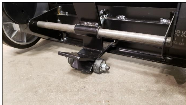
FIG. 10.1 – FOOT BRAKE ON NON-STAIRCLIMBING UNITS
