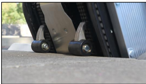
FIG. 6.3 - LIFTING FEET PLACED ON STEP
