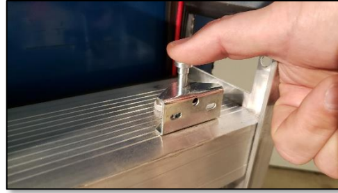
FIG. 6.2 – REWIND LOCK PIN
