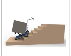
The CT250/300/250A/300A will go up slowly before the tracks leave the ground completely. When CT250/300/250A/300A is in the automatic mode to automatically adjust the loading board Angle, the running speed of the track will be automatically reduced.
