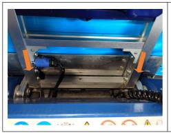
Insert the aluminum alloy vertical beam of CT250A/300A into the corresponding slot on the machine base.
