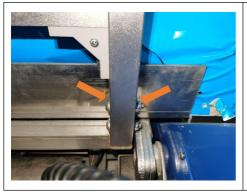
Install the alloy vertical beam in the installation position using the screws, gaskets and lock nuts.
