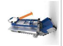
Open the steel back support of the CT250/300 to vertical Angle.
