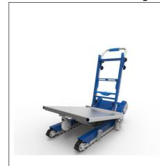
The CT250/300/250A/300A can walk on flat ground with crawler tracks. Switch to the Loading board control mode, raise the loading board to an angle till the crawler tracks touch the ground, and then switch to the track mode and walk by the crawler tracks. This way is applied to short distance walk or on uneven road surfaces.
